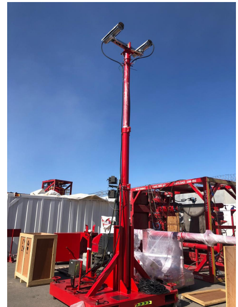
Thermal Camera mast
