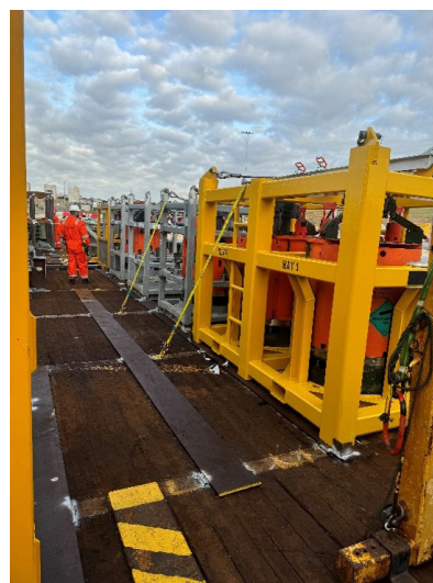
DSV back deck working area with two Catcher SCM's located in the deployment frame (foreground of photo) and transit frames in background housing spare Catcher SCM's
